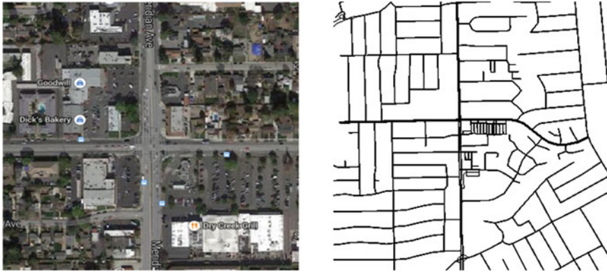
Fig. 6 San Jose (California) urban area captured from Google Maps ( left ) and exported to a VANET network topology by using MOVE/SUMO ( right )
