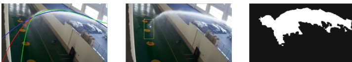
(e) jet fitting (f)location of the water points (g)the traditional method for jet region extraction
