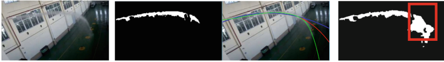
(a)original image (b) matching image(c)fitting curve (d)the traditional method for jet extraction
