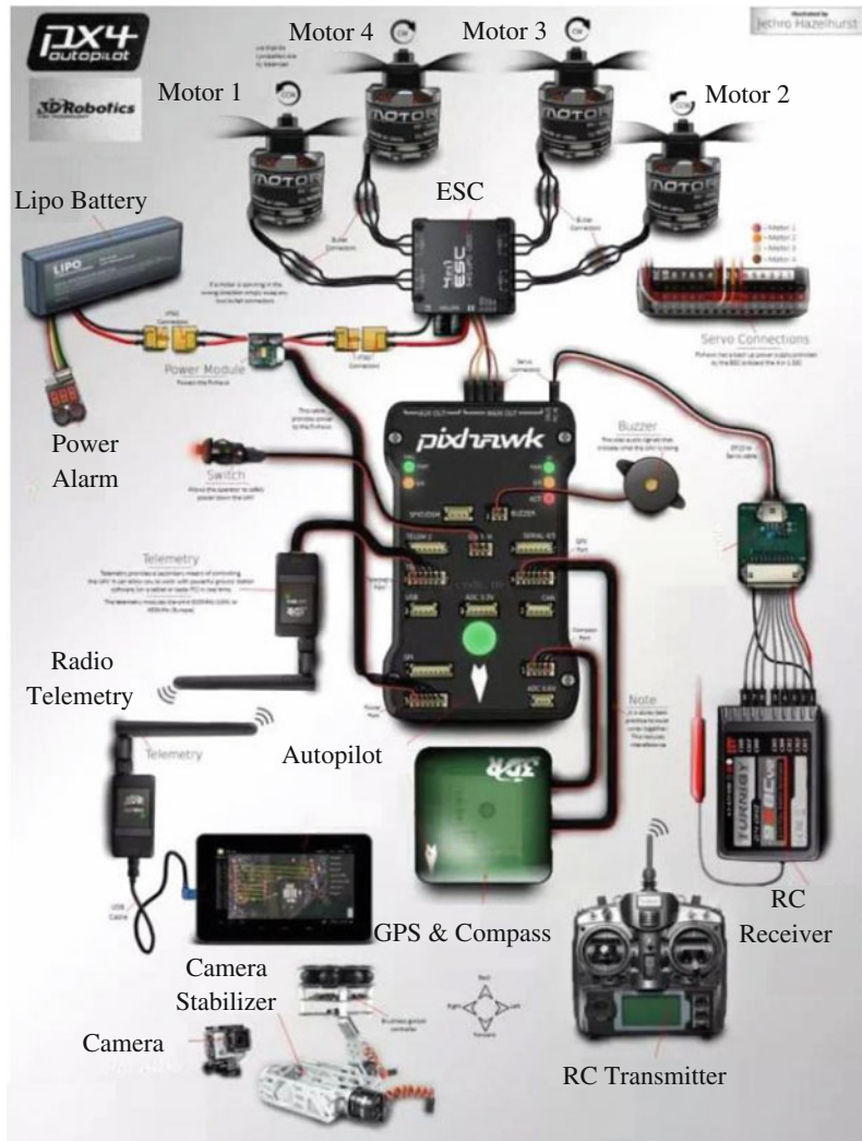
Fig. 2.2 Combination and connection of a multicopter system (photo by Jethro Hazelhurst from http://www.ardupilot.org )
