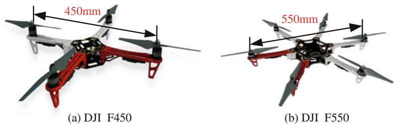
Fig. 2.5 Diagonal size of multicopters
