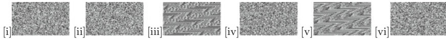
Fig. 1 Pictorial representation of ciphertext corresponding to different quasigroup constructions applied to trivial data with a trivial key: i Resultant Ciphertext using (nonlinear) PQG1, ii Resultant Ciphertext using (nonlinear) PQG2, iii Resultant Ciphertext using third (linear) PQG3, iv Resultant Ciphertext using (linear) PQG4, v Resultant Ciphertext using (linear) PQG5, vi Resultant Ciphertext using generalized (linear) PQG6 of Sect. 1
