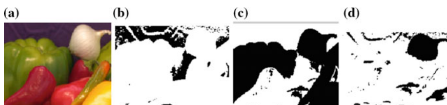
Fig. 2 a Original RGB image. b Masked red image. c Masked green image. d Masked blue image
