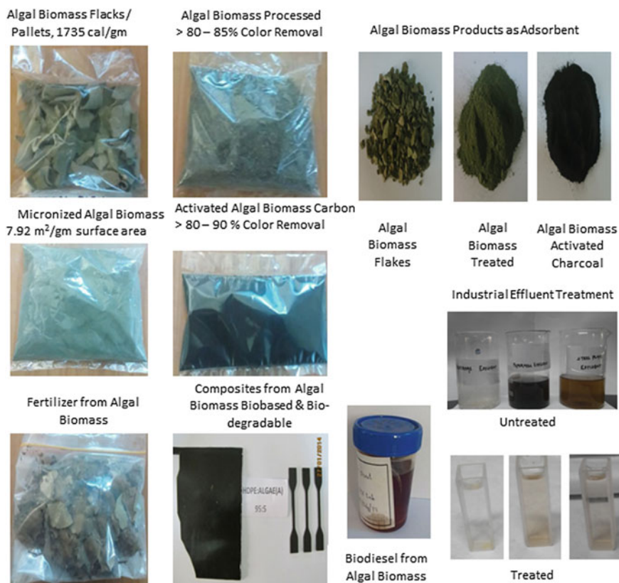
Fig. 2 Products from carbon sequestration plant
