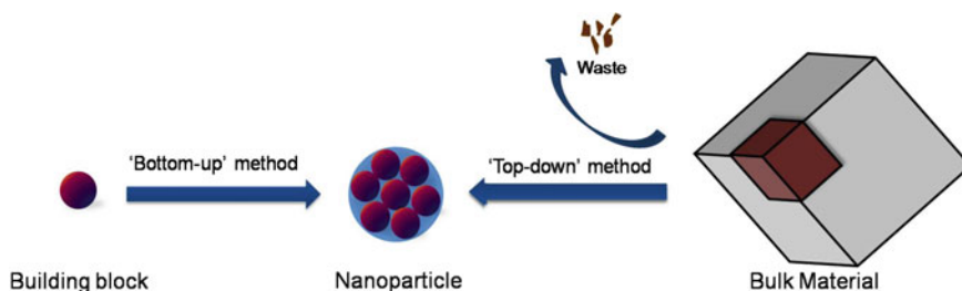
Fig. 1 Synthesis of nanoparticles; the 'Bottom-up' method recruits atoms and molecules in the aggregated nanoparticle form. The 'Top-up' method involves sculpting of bulk material which also generates high waste in comparison to bottom-up method
