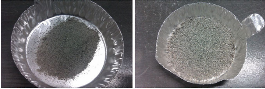
Fig. 12.1 Photograph of municipal solid waste incinerator bottom ash ( left ) before and ( right ) after carbonation
