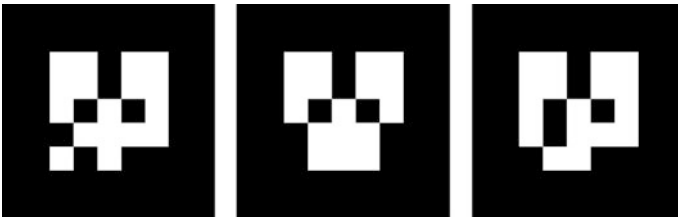
Fig. 2 AR marker tags used for image based visual servoing
