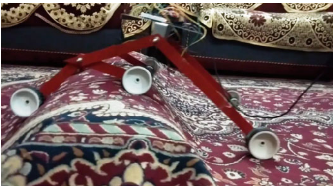
Fig. 2 Rocker bogie rover on undulating surface
