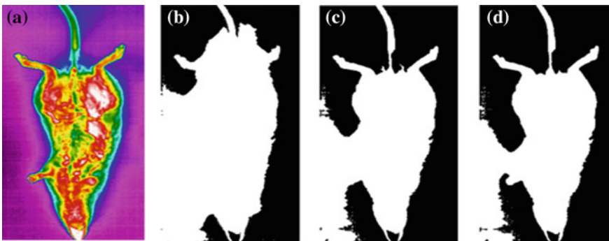
Fig. 8 Thermal image segmentation using the Active Contour method including a the raw thermal image b after 300 iterations c after 600 iterations and d after 700 iterations
