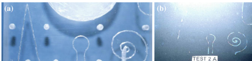
Fig. 4 Plexiglas phantom with thermoresistors to measure the acquisition time of the correct image [9] (Reprinted from Montruccoli GC, Montruccoli Salmi D, Casali F. A new type of breast contact thermography plate: a preliminary and qualitative investigation of its potentiality on phantoms. Phys Medica 2004; XX(1):27–31, with permission from Elsevier. doi: 10.1400/19286 )
