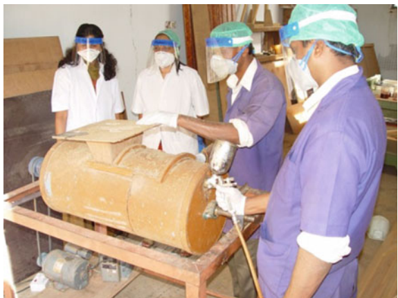
Fig. 5 Spraying of resin to the fibres
