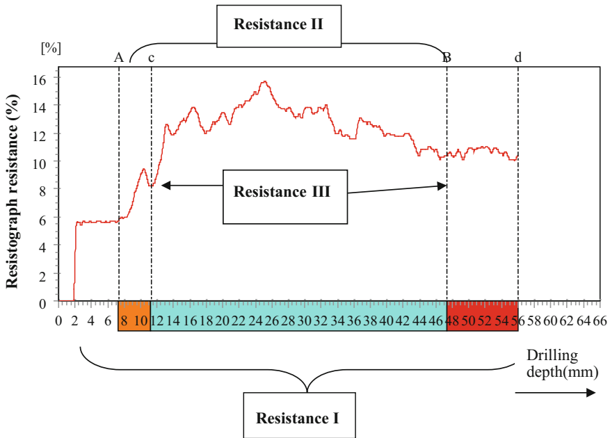
Fig. 1 Resistograph profile at different regions, namely, whole reading ( resistance I ), truncated with bark to pith ( resistance II ) and without bark ( resistance III )
