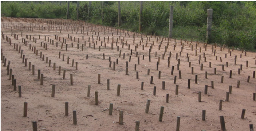
Fig. 1 Exposure of preservative specimens in the test yard
