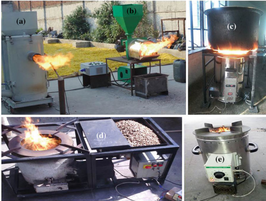
Fig. 2 Pellets based eco-equipment. a Industrial pellet burner b Green burner c SMART cooking stove d Continuous feeding stove (CFS) e ATOM cook stove
