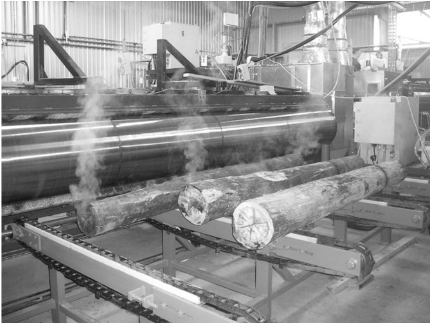
Plate 2 Continuous 300 kW pilot microwave processing of poles
