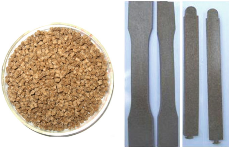
Fig. 1 Lantana–PP composite pellets and test specimens
