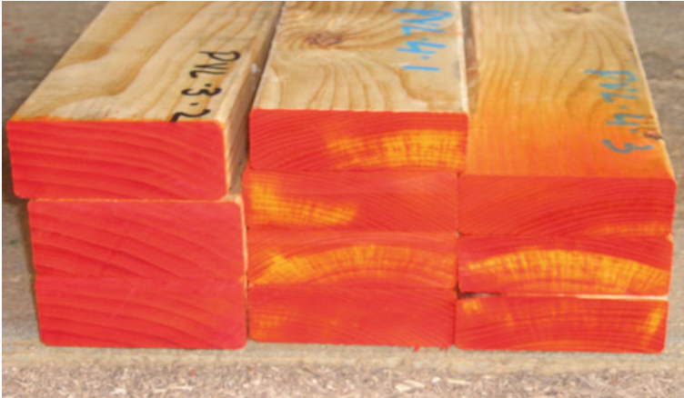
Plate 5 Framing timber spot tested for boron preservative. There is full sapwood penetration ( red colour ) and incomplete heartwood penetration ( yellow )
