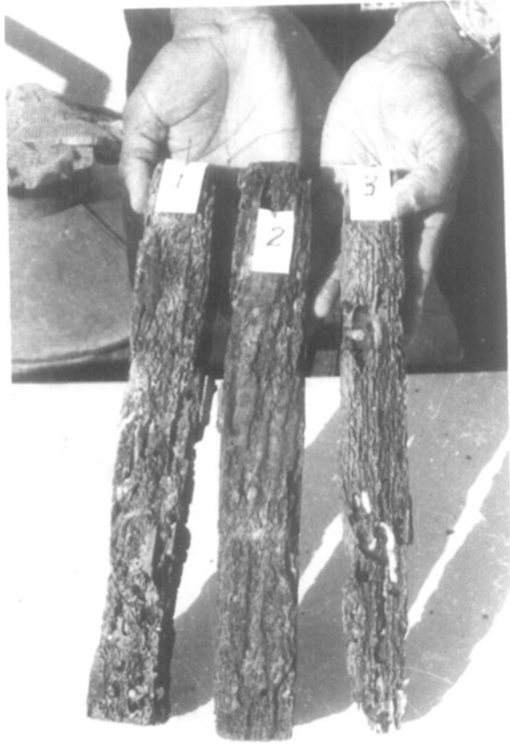
Fig. 2 Severe surface destruction of wooden test panels by Limnoria within eighteen months. (Locality: Mumbai Harbour)
