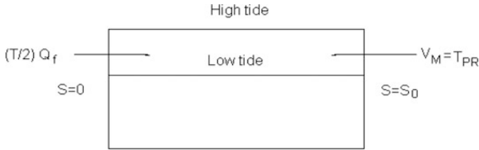
Fig. 6.3 Schematic diagram of the tidal prism model. Water exchanges and the salinities at the boundaries are indicated. For convenience the tidal prism ( T_{PR} ) will also be denoted by V_M
