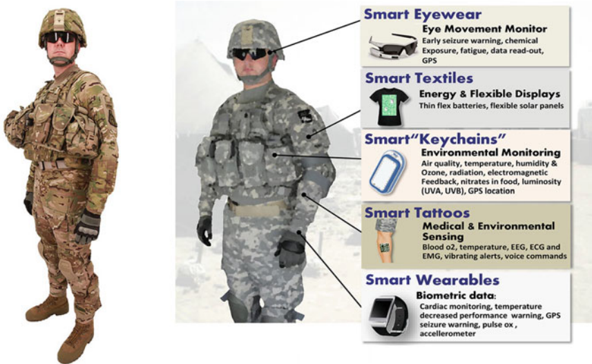
Fig. 2.10 a A soldier equipped with different SNs [6] and b closer look at a soldier with different SNs [7]
