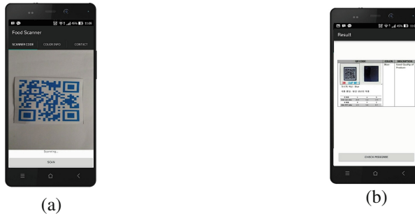
Fig. 4. (a) The app scanned the TTI QR code based and (b) shows the product quality based on its color
