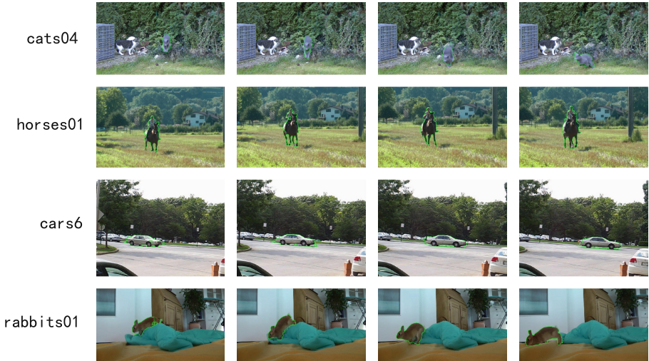
Fig. 7. Some segmentation results on FBMS dataset. The regions within green boundaries are the segmented foreground objects. (Color figure online)
