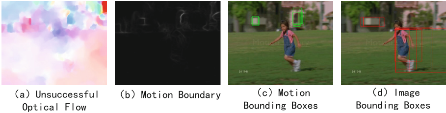
Fig. 2. (a) A failing case of optical flow. (b) Motion boundary. The motion boundary fails following the optical flow. (c) Some top ranked motion bounding boxes. The motion bounding boxes are outside of the target. (d) Some top ranked image bounding boxes.
