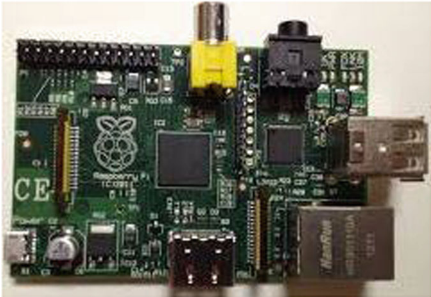
Fig. 24.3 Top side view of Raspberry Pi board
