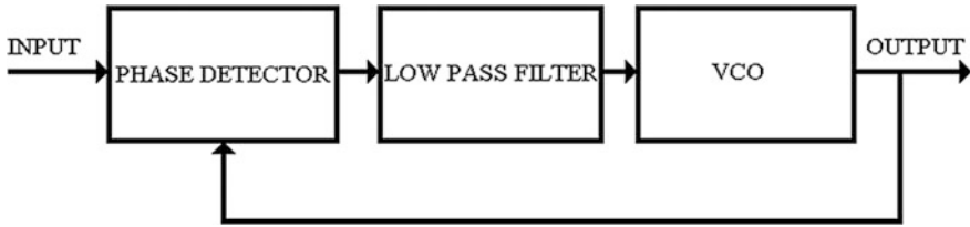
Fig. 30.1 Top-level block diagram of a Phase-Locked-Loop circuit
