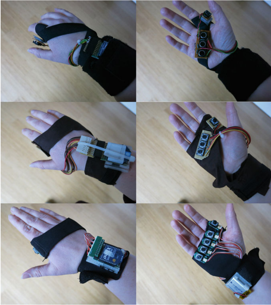
Fig. 2 The three stages in the development of the gestural controllers of “Wezen—Gewording”. At the top the first version, middle the second, and bottom the final version
