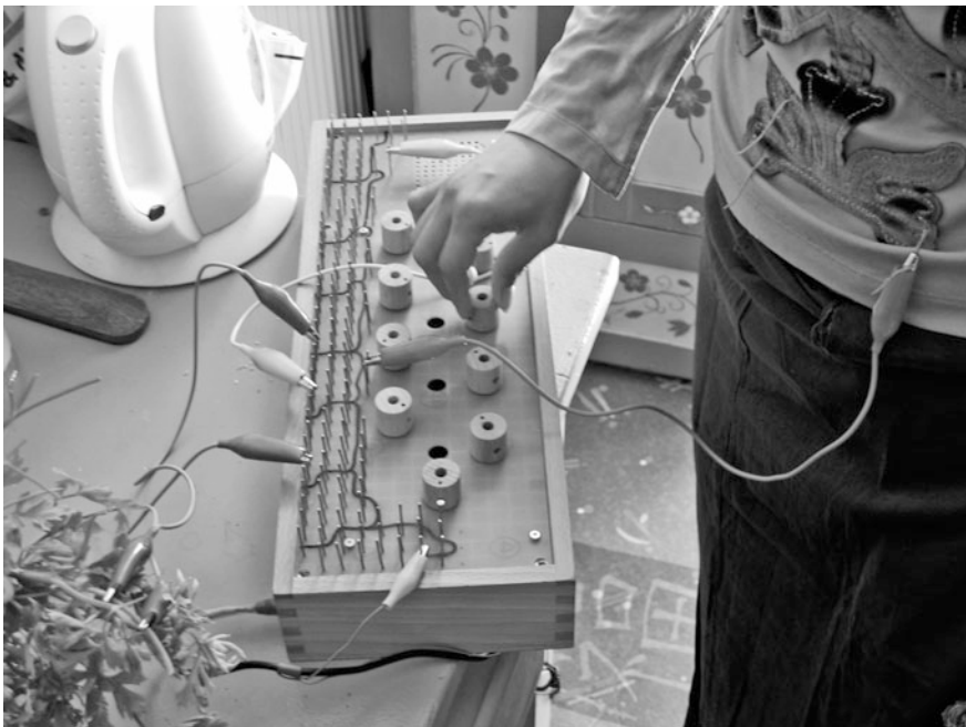
Fig. 2 Echo Ho performing a kitchen concert on a Blasser KitTenNetTik synthesizer kit assembled by Ralf Schreiber. The 100+ metal rod electrodes are the “androgynous nodes”, connected by alligator clips to vegetables and body contacts. Image © Hannes Hoelzl 2006
