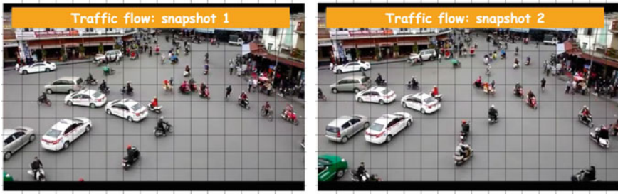
Fig. 8.2 Two subsequent snapshots of traffic flow in Hanoi separated by a sub-second time-interval, overlaid with a uniform grid in the field of view. (Source http://www.YouTube.com .)
