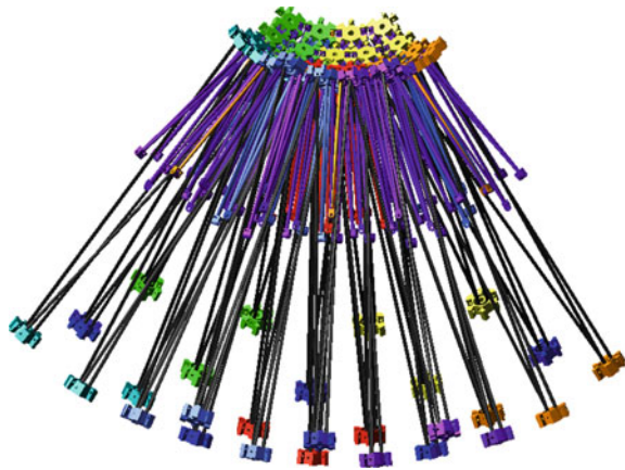
Fig. 12 Folded configuration of the antenna
