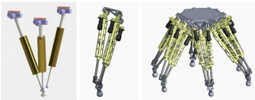
Fig. 2 Leg model of R-P in 3-active-parallel limbs and the six-legged robot
