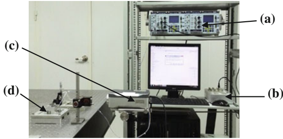
Fig. 4 The experiment system of stick-slip actuated structure. a Controller of piezoelectric ceramic. b dSPACE 1104, which can convert the digital control signal into analog signal. c Laser interferometer, the measurement accuracy is 1 nm. d The prototype of stick-slip actuated structure
