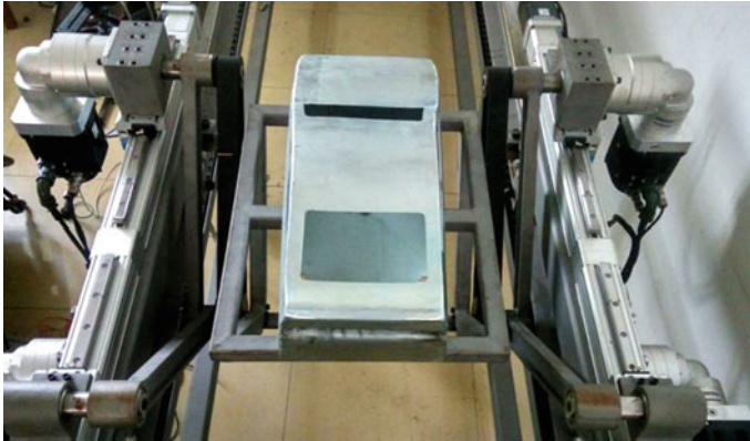
Fig. 6 Electro-coating conveyor with two same parallel mechanisms
