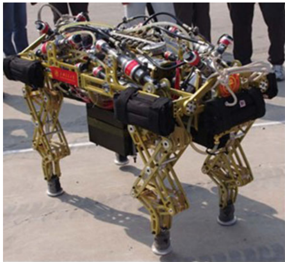
Fig. 1 The baby elephant robot with hydraulic pump is design to carry high payload. It has decoupled design of the motion and the power
