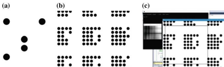
Fig. 9 Using template matching algorithm to find dot array
