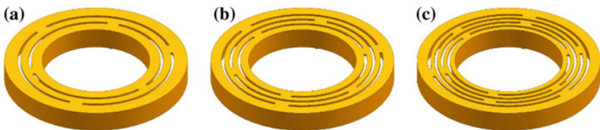
Fig. 3 The conceptual model of silt diaphragm flexure. a 1 \times 3 type, b 2 \times 3 type, c 3 \times 3 type
