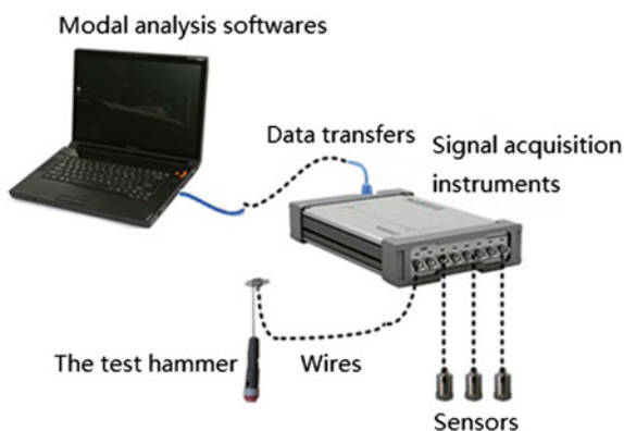
Fig. 3 The sketch of the connection of experimental equipment
