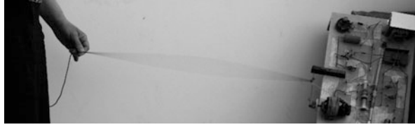
Photo 6.2 Fundamental or first harmonic
