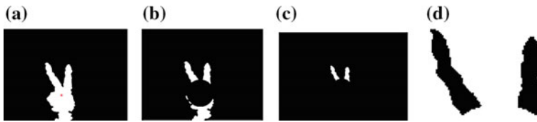
Fig. 5 a Image with centroid of the hand, b image with circle drawn from centroid with minor axis diameter, c non-finger components are removed from image, d fingers cropped from the image
