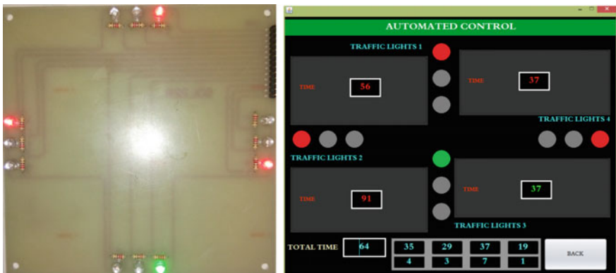
Fig. 12 Intelligent traffic signal management system (Hardware and GUI)
