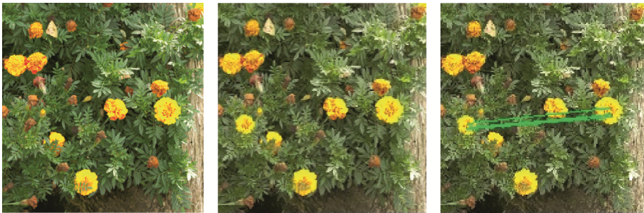
Fig. 3. Original image, forged image (cloned region scaled) and forgery detected using ACC.
