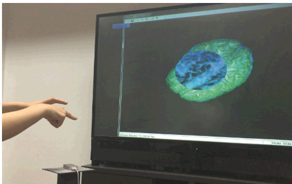
Fig. 8. Bimanual gesture interaction with the MRI human brain volume model
