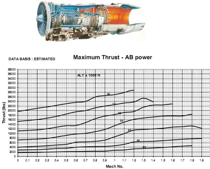
Fig. 1. Thrust curve of engine F100-PW-200
