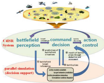
Fig. 1. The conceptual schematic of parallel simulation for the command decision support
