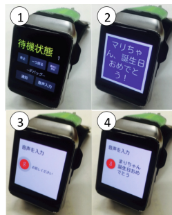
Fig. 4. Screens of smart watch. 1. Stand-by screen; 2. Lines screen; 3. Voice input screen; and 4. Input result screen
