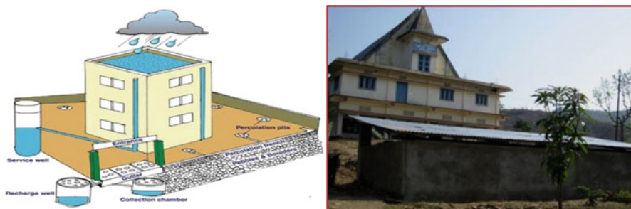
Fig. 16.9 Rooftop water-harvesting structure at Mon
