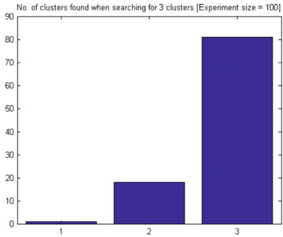
Fig. 2 A count of number of clusters created over 100 runs of normal k-means
