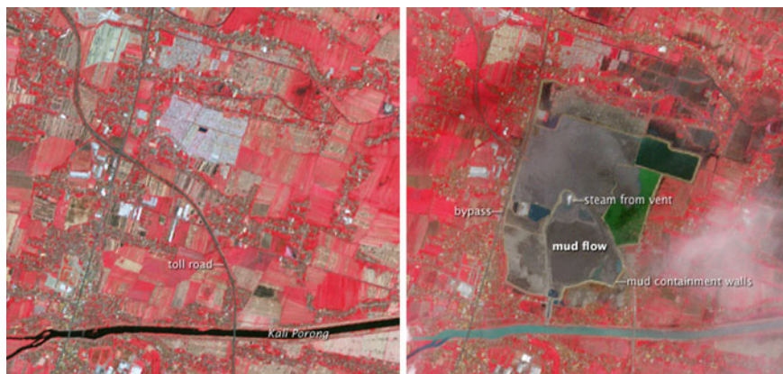
Fig. 9 NASA's Aster false color composite before ( left ) and after ( right ) the eruption of the mud volcano Lusi at Sdiaoarjo, Indonesia, the biggest mud volcano of the world. The vent is suspected to have resulted from drilling-induced fracturing at the site ( Source Wikipedia)
