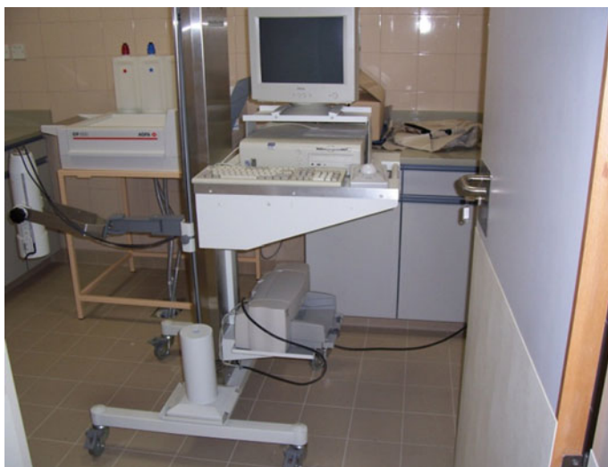
Fig. 5 Well counting system for estimation of I-131 activity/mL
