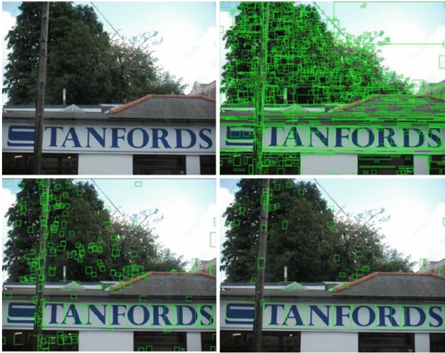
Fig. 3 Result after character descriptor (from the left to right are original map, map after MSERs detection, result of coarse classifier, map after neural network classifier)
