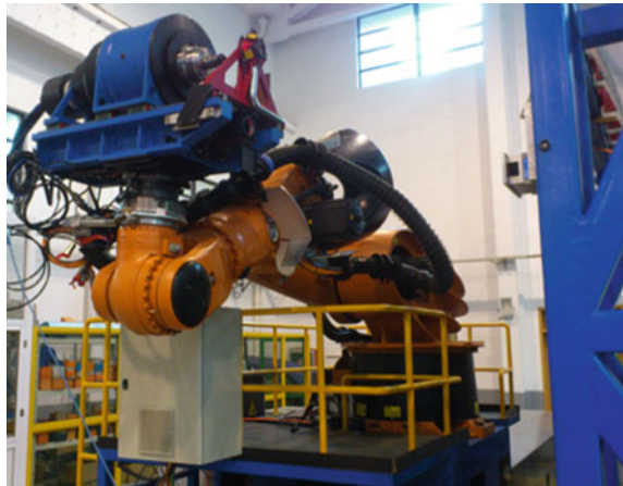
Fig. 1 ZJU's robotic drilling system equipped with a vision system
