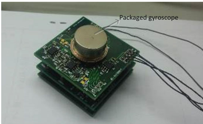
Fig. 8 Vacuum packaged gyroscope with PCB test circuits
