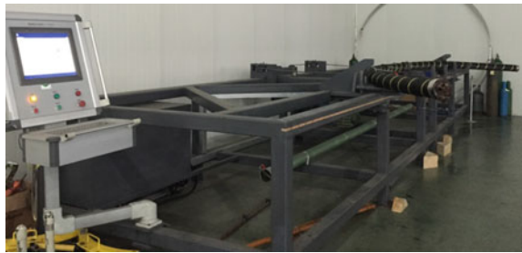
Fig. 6 Automatic bending stiffness testing system
