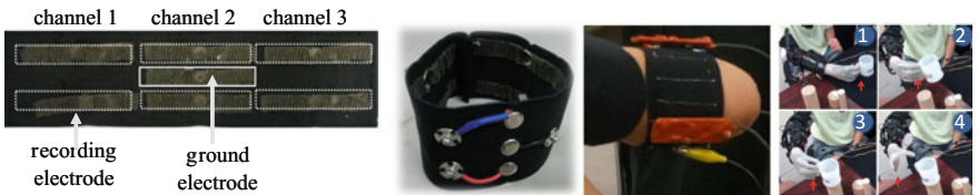
Fig. 2 PPy-electrode sEMG sensor band ( left ) and two subjects wearing sensor bands customized for them ( middle and right )
