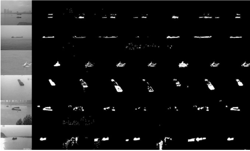
Fig. 4 Comparative results on six video sequences. From left to right: test frame, ground truth, GMM, ViBe, LOBSTER, AdaDGS, GMCA, ours, respectively
