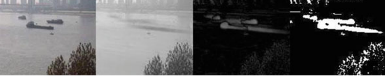
Fig. 1 Results of background subtraction based on compressive sensing. From left to right: original frame, background, foreground, background-foreground binary image
