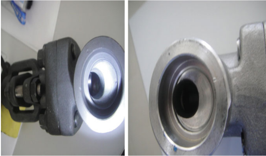
Fig. 4 Surface and debris inside the valve
