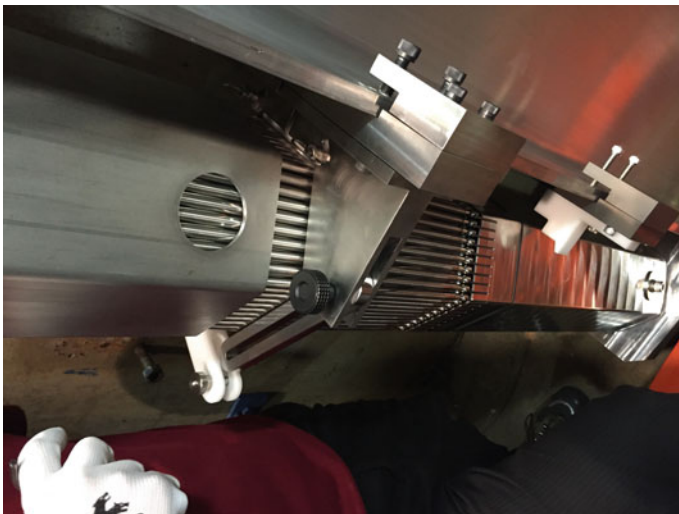
Fig. 2 TerraPower mock-up fuel assembly with wire-wrapped pins and wrapper/duct
