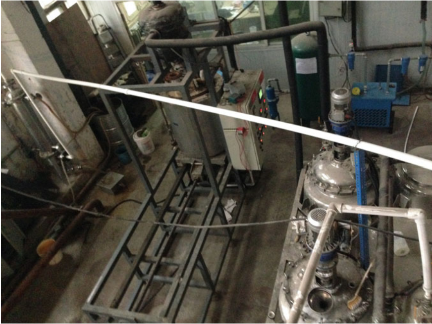
Fig. 6 The in-drum drying prototype device of concentrates
