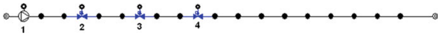
Fig. 2 Calculation model of single feedwater line: 1 feedwater pump; 2 feedwater control valve; 3 feedwater isolation valve; 4 feedwater check valve
