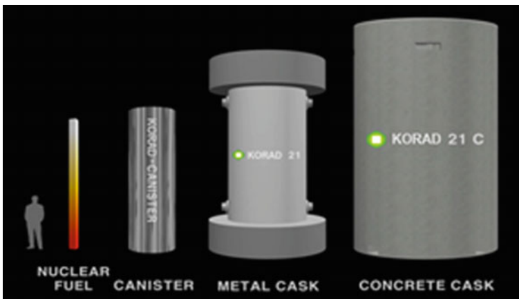
Fig. 1 Design concept of concrete cask storage system
