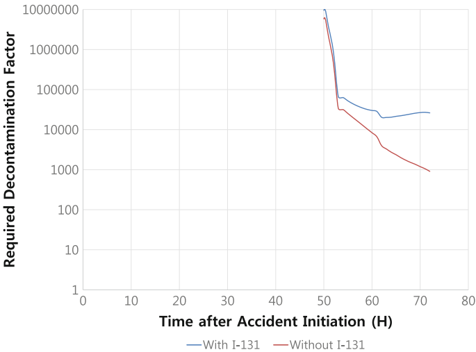
Fig. 12 Required decontamination factor versus time
