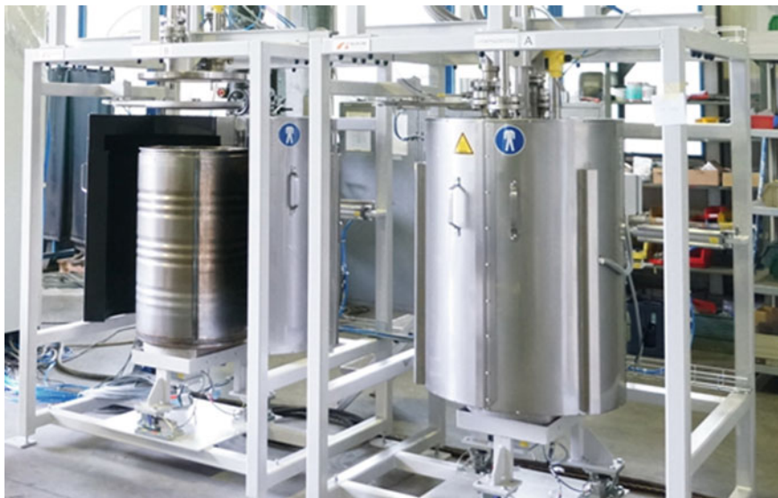
Fig. 4 Equipment photograph of still residue in-drum dryer
