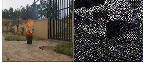
(a) original picture (b) gradient image based on Sobel operators (the size of core is 5*5)
