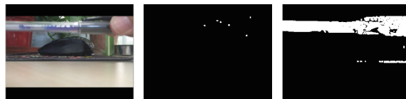
(c1) original pictures; (c2) GMM based on 3 \times 3 core gradients; (c3) GMM based on RGB
