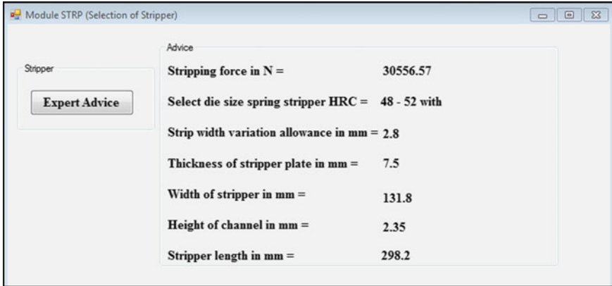
Fig. 15 Output of STRP module for example part
