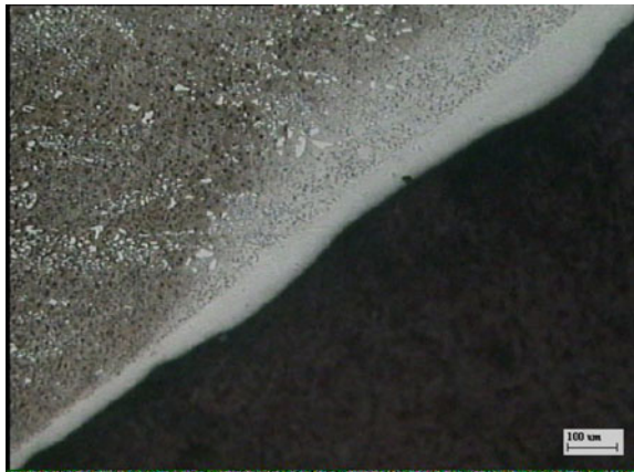
Fig. 23.46 Micrograph of the outer surface of the inner race showing a white-etching layer (etchant: 2 % nital) (100 \times )
