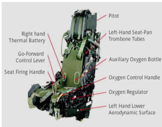
Fig. 13.9 Military aircraft ejection seat
