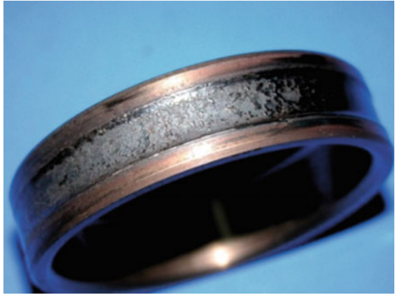
Fig. 23.44 Badly worn outer surface of the inner race of the bearing (1.25 \times )
