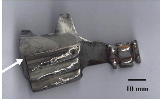
Fig. 23.25 Fracture surface of the failed inner gear showing the fracture profile characteristics and the origin (arrowed)
