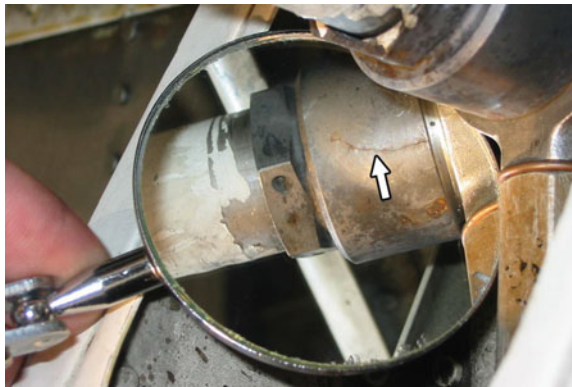
Fig. 19.5 SCC (arrowed) in a 431 nut
