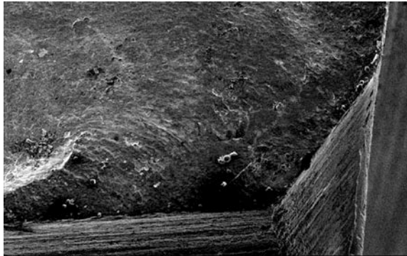
Fig. 23.26 SEM fractograph of the fracture surface showing the origin at the tooth root fillet and (very) faint progression markings (50 \times )
