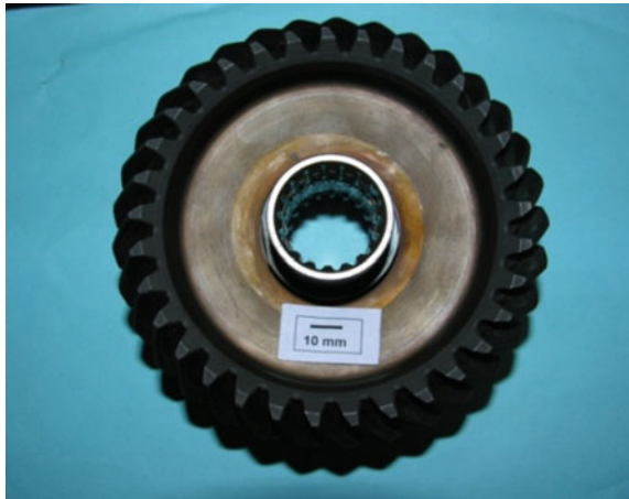
Fig. 23.18 The failed HPCR gear received for examination
