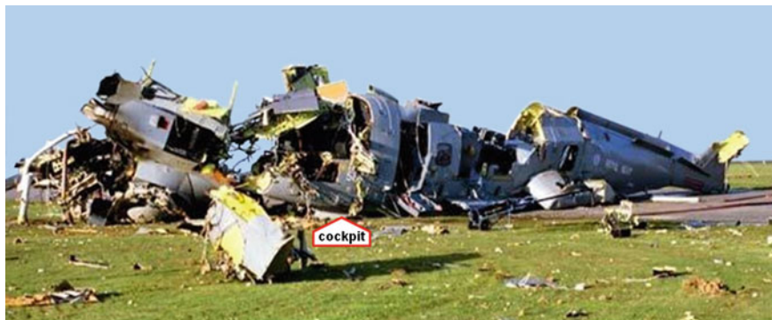
Fig. 18.2 Disintegration of the Merlin helicopter owing to a fall from 4–5 m [12]
