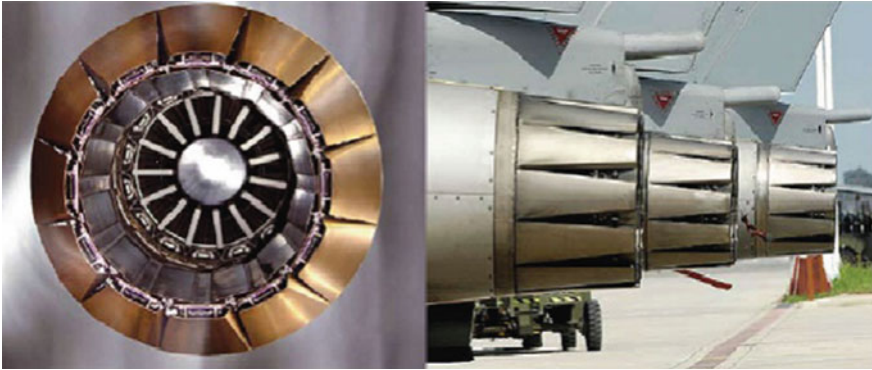
Fig. 3.13 Rear and side views of an SPF Ti-6Al-4V exhaust nozzle used for EJ-200 engines [103]
