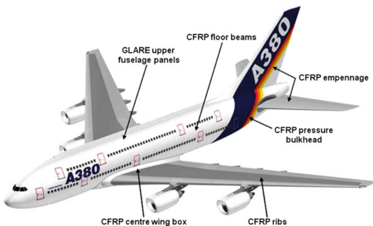
Fig. 8.6 GLARE (GLASS REinforced aluminium laminates) and CFRP components in the Airbus A380: see Chaps. 13 and 14 in Volume 1 of these Source Books
