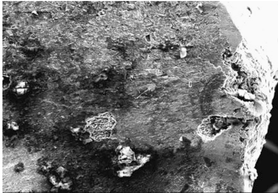
Fig. 23.16 SEM fractograph showing pitting corrosion at the leading edge of the blade (two irregular pits just on the 'nose' of the leading edge) (200×)
