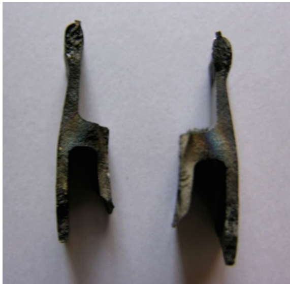
Fig. 23.35 Fracture surfaces after opening the primary crack (0.5×)
