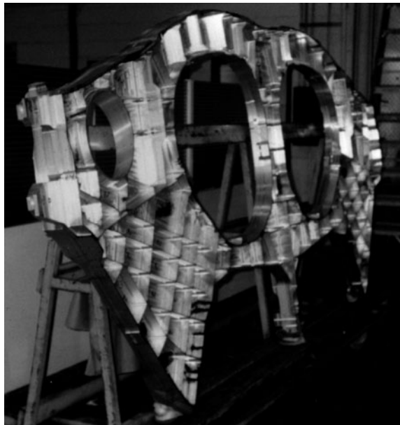
Fig. 6.11 Machined bulkhead forging for a twin engine military aircraft, [1]
