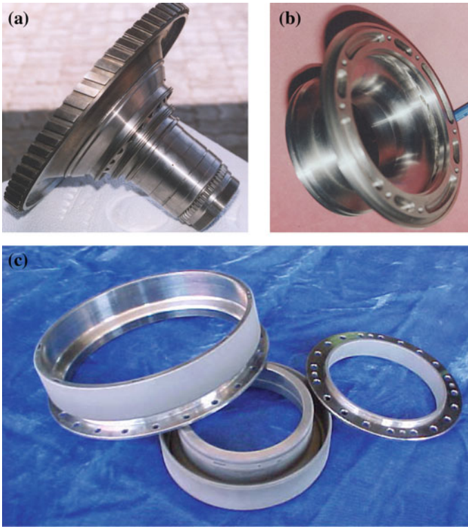
Fig. 22.6 a WC-17Co coated compressor disc and b-c WC-12Co coated nozzle parts
