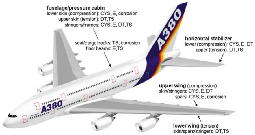
Fig. 2.7 Engineering property requirements for main structural areas in a transport aircraft: CYS compressive yield strength; E elastic modulus; TS tensile strength; DT damage tolerance properties (fatigue, fatigue crack growth, fracture toughness)
