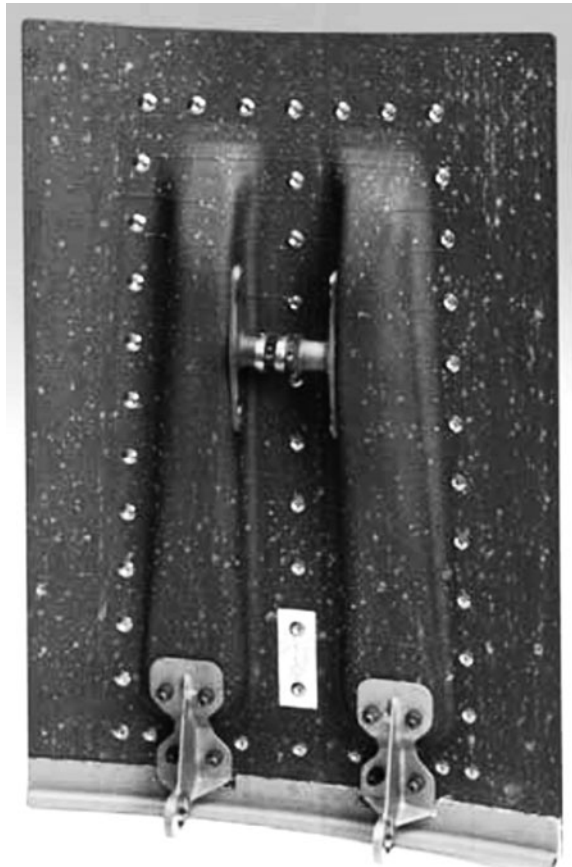
Fig. 16.9 C-SiC composites for thermal protection systems (TPS)
