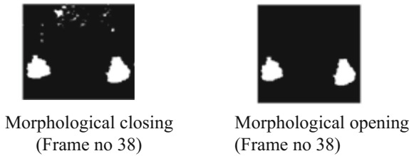
Fig. 6 Foreground extraction using background subtraction
