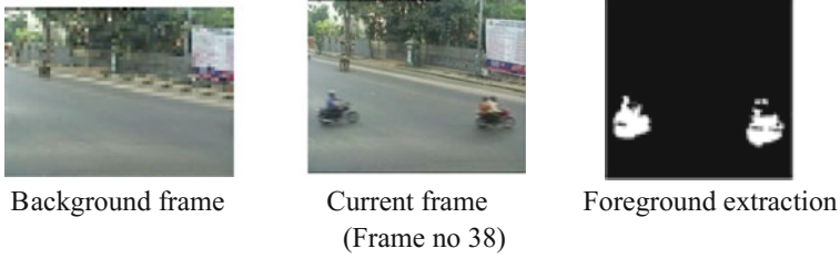
Fig. 6 Foreground extraction using background subtraction
