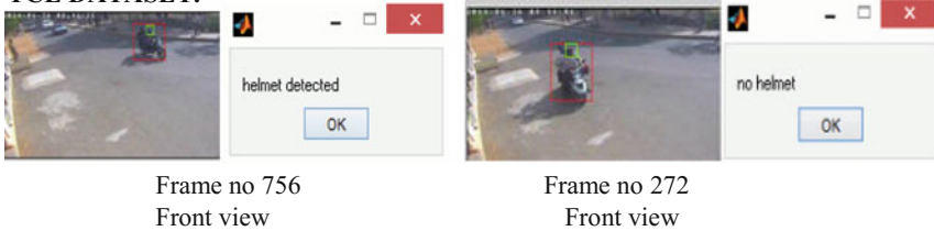
Fig. 9 Motorcyclist wears helmet or not classification using KNN classifier for TCE dataset
