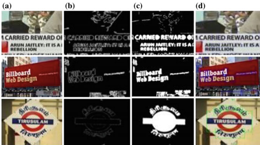
Fig. 2 Output for each stage: a Input image. b Edge detection. c Stroke width transformation. d Output
