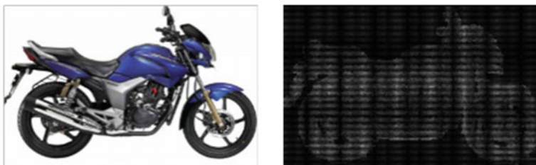
Fig. 2 Extracted HOG features for an input frame
