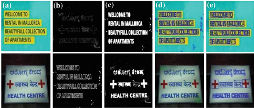
Fig. 6 Output script independent text segmentation. a Input image. b Edge detection. c Stroke width transformation. d Initial text regions. e Output image
