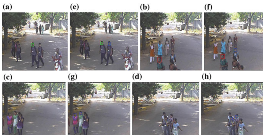
Fig. 5 a–d Face detection using Viola Jones Dataset: College dataset Frame size: 704 \times 576 and e–h Face detection in de-blurred frame Dataset: College dataset Frame size: 704 \times 576
