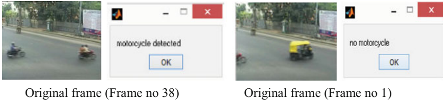
Fig. 5 Motorcycle detection and verification using KNN classifier
