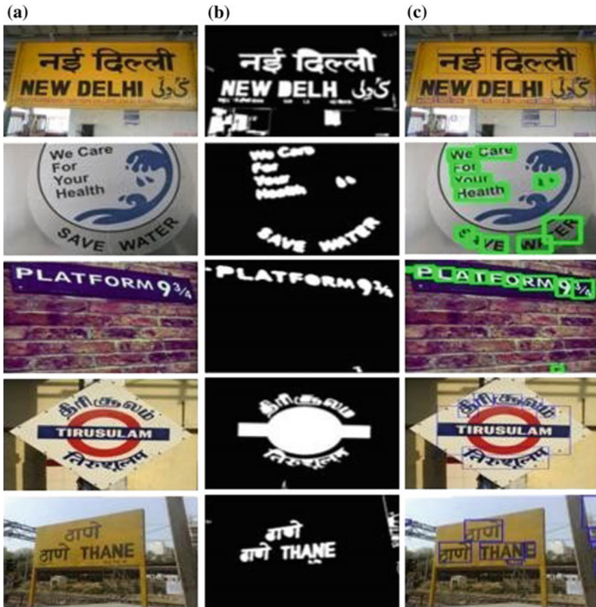
Fig. 9 Output for multi-oriented script independent text segmentation. a Input image. b Text regions. c Output Image
