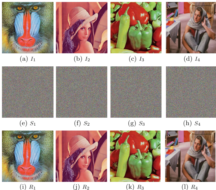
Fig. 3 Proposed scheme of (n, n) -MSIS scheme for colored images with n = 4 : a–d Secret images ( I_1, I_2, I_3, I_4 ). e–h Shared images ( S_1, S_2, S_3, S_4 ). i–l Recovered images ( R_1, R_2, R_3, R_4 )
