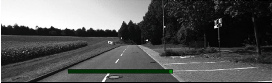
Fig. 8 Line scanning of the road surface
