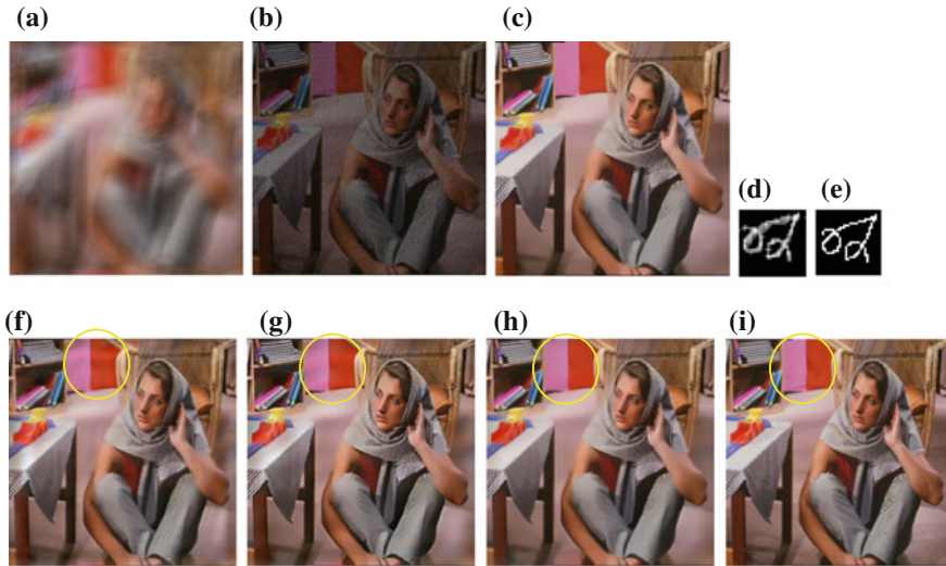
Fig. 6 a Blurred image. b Input noisy image. c Denoised image after exposure correction in noisy image. d Estimated kernel. e Actual kernel. f RL output (PSNR = 24.42). g Algebraic deconvolution (PSNR = 22.69). h BPD output (PSNR = 26.40). i Original image
