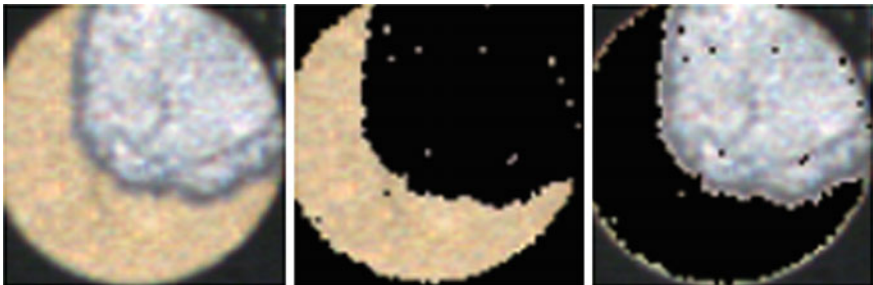
Fig. 3 Defect image, Copper part, Non-copper part C
