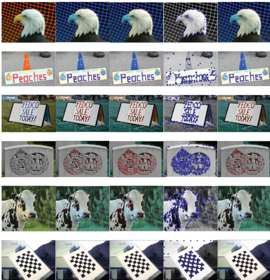
Fig. 4 First column—original images, corners detected using: second column—Harris corner detector [4], third column—FAST corner detector [8] fourth column—SUSAN [7], fifth column—proposed method
