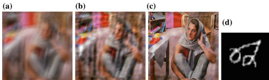
Fig. 3 a Blurry image. b Deconvolution without the residual image concept. c Deconvolution with the residual image concept. d Estimated kernel
