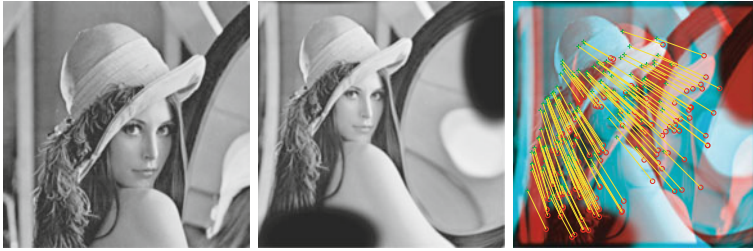
Fig. 1 An example of set of spatial correspondences obtained from moving image Lena that undergoes a pin-cushion-type deformation
