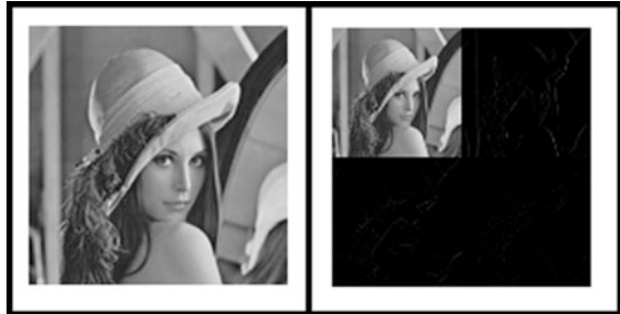
Fig. 3 Example of applying Haar wavelet (original image of Lena— Left and image produced by Haar wavelet transform— Right )
