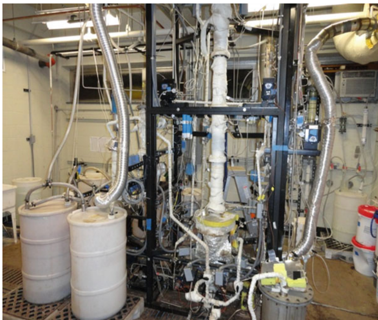
Fig. 3.3 The continuous-operation Sequential Liquid-Lignin Recovery and Purification (SLRP) unit at Clemson University, USA
