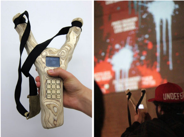
Fig. 2 The movable interface SMSlingshot by VR/Urban. Right person shooting a message to a façade
